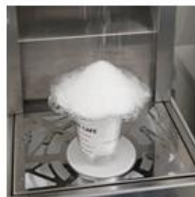
Automatic turn table for properly shaped ice
