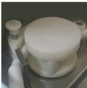
Suction Pump and sensor for automatic ingredient input
